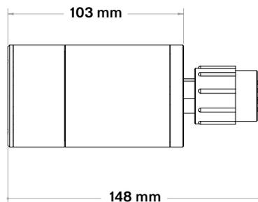
(Somewhat) larger package, loads more power. Whether your deployment involves a mid-sized ROV, a USV (overboard camera), or a simple stand-alone inspection, some missions call for nothing less than the *Artemis-Puffin*. At 60 mm in diameter, the Puffin boasts all the capabilities of the Auk, with the addition of four (4) built-in LED light modules. As remarkably simple and durable as any Reach camera system, the Puffin is rated for operation at depths of up to 300 meters.
