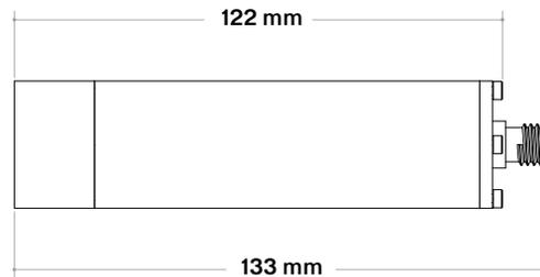
Don't let its size fool you. With a diameter of just 32 mm and a length of 122 mm, the *Artemis-Auk* delivers exceptional quality and performance under even the most challenging remote monitoring & inspection conditions — in the air, on the ground, and up to 2,000 meters underwater. Robust and reliable, it attaches to your inspection class ROVs to provide HD auxiliary video, or combines with a separate LED light to create a complete commercial diver camera package.
